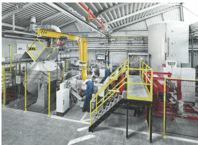
The semi-industrial direct chill casting machine for horizontal continuous casting of aluminium alloys with real time control unit at the AIT.
